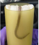
Tape over the end of the micro-CT sample holder to ensure that nothing protrudes from the sample holder and label the tape with the mouse ID written on the Falcon tube that the mouse was stored in. Flatten the tape on the sample holder as much as possible.
