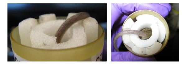
Tuck the tail into the micro-CT holder on the outside of the foam.
